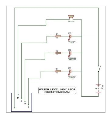
Fig.4.1 Water Level Indicator Circuit
